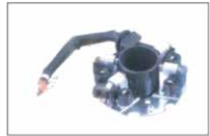
CB-8181 Brush Holder Assy Use for: Mitsubishi PMGR Starters Spec:4.5×18×17.5
